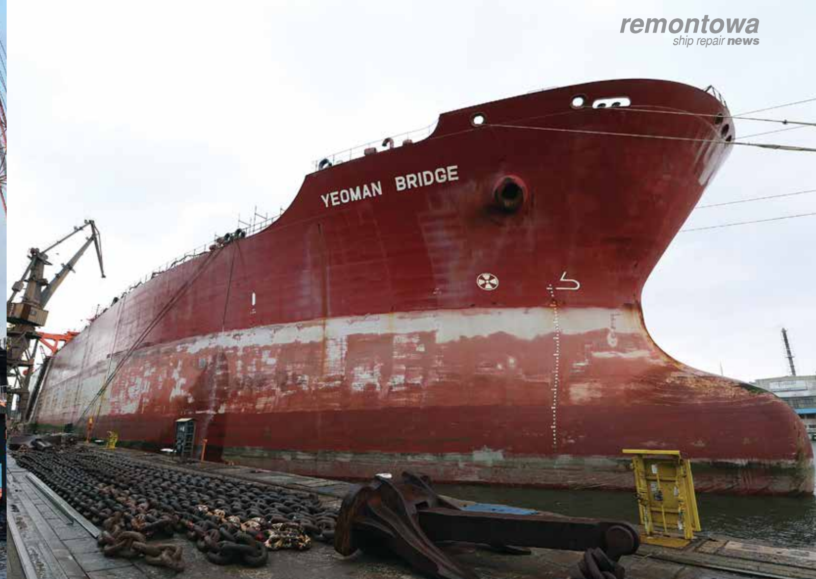
Almost 9 tons of steel being internal structure and external sheathing was exchanged on the Yeoman Bridge self-discharging bulk carrier. Photo: Sławomir Lewandowski
