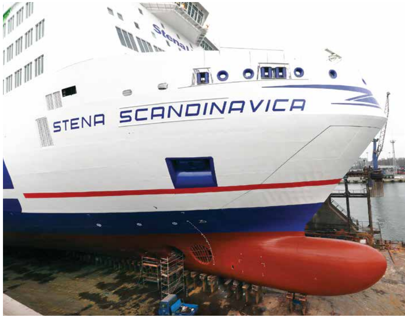
Apart from being retrofitted with scrubber, the ferry has received silicone coatings applied on its hull. Photo: Slawomir Lewandowski
