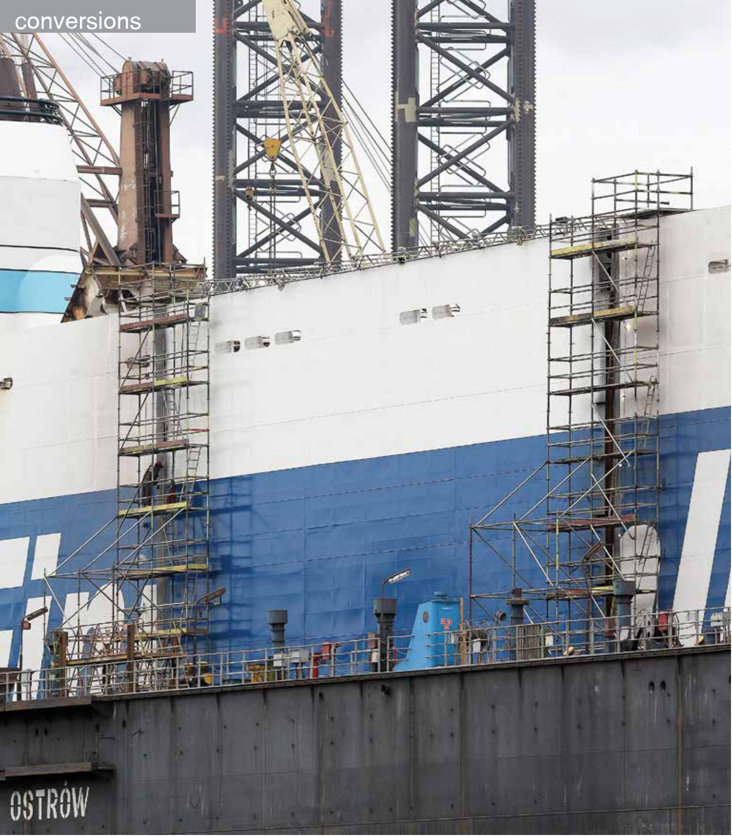
The steel insert before being welded and integrated into the ship's hull. Photo: Sławomir Lewandowski
