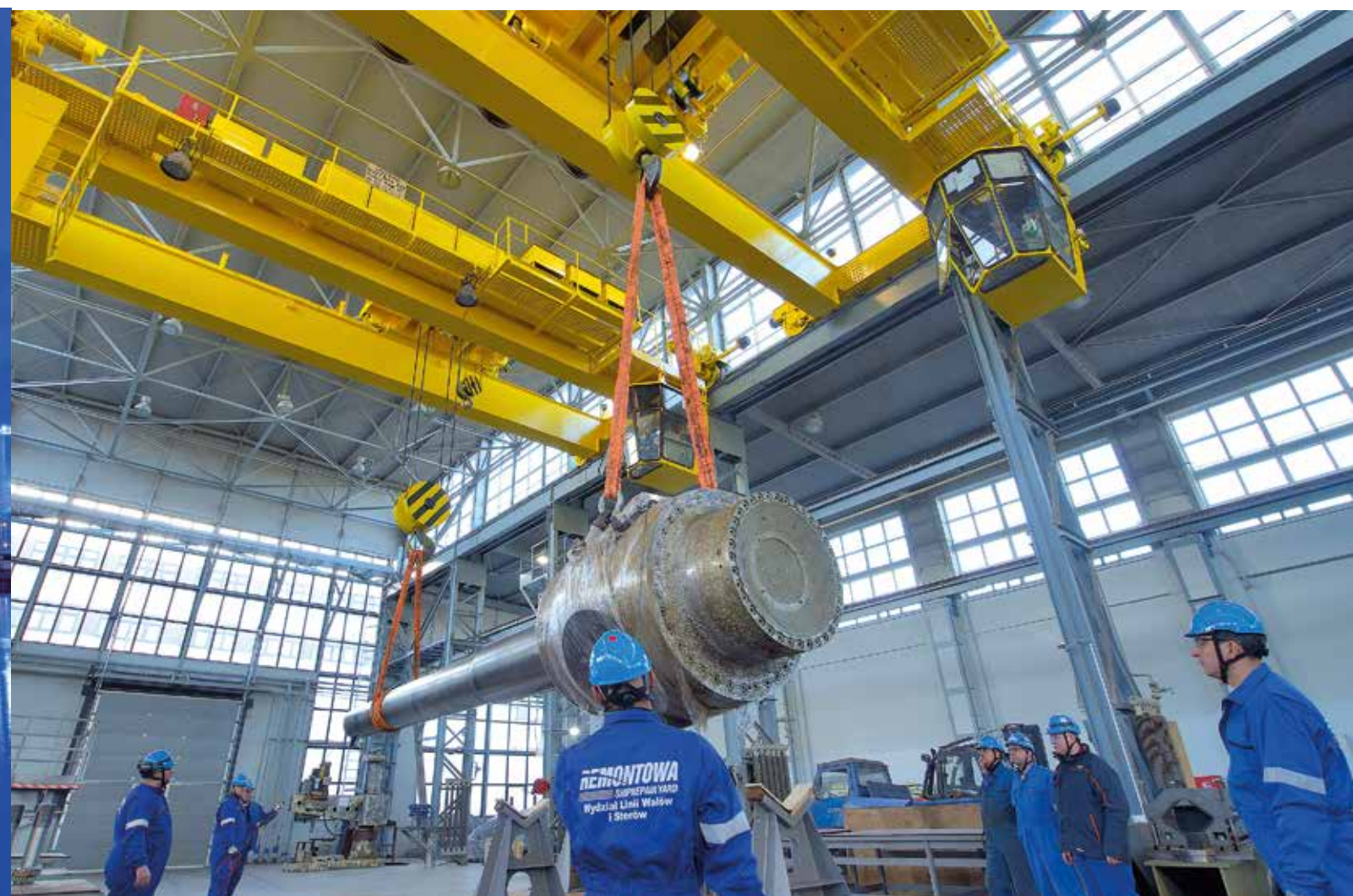
Its propeller shaft line underwent an overhaul in the modernized hall of the Marine Power Plant Department. Photo: Remontowa SA
