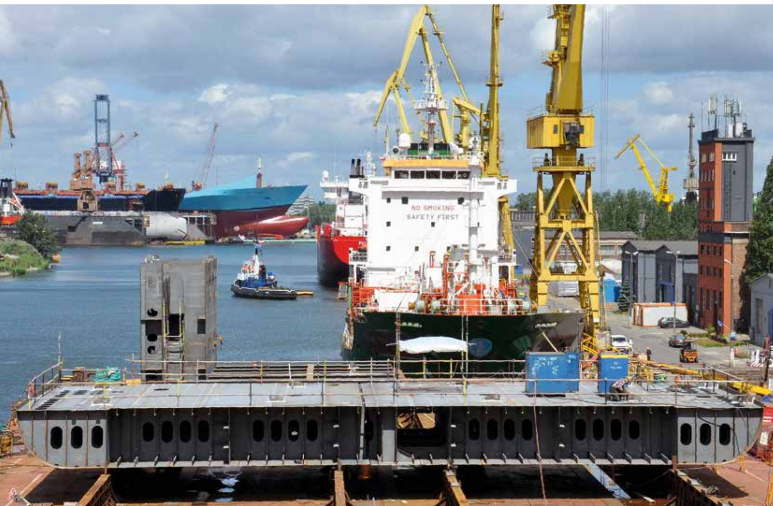
The first steel section weighing 55 t for the insert destined for Finntide was laid onboard the semi-submersible barge REM LIFT 24000 on the 29th of June 2017.
