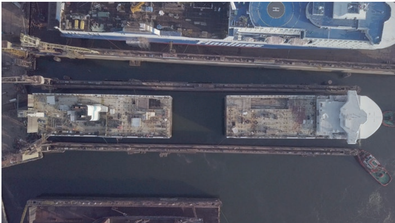
The ship's hull cut and divided into two parts...
