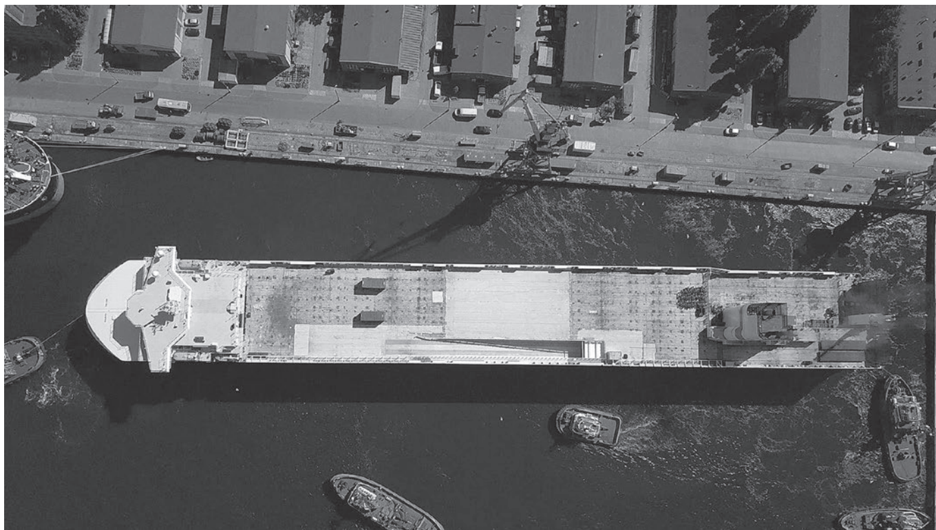
Finnsun with the steel insert welded and integrated into the ship's hull. Photo: Marcin Koszałka
