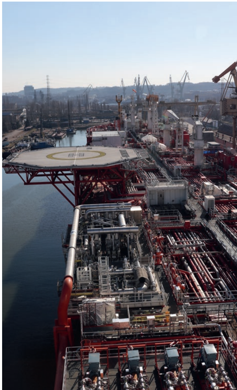
A glance at the ship's deck. More than 30 km of tubing and over 400 km of cables were laid on the FSO at Remontowa SA.
