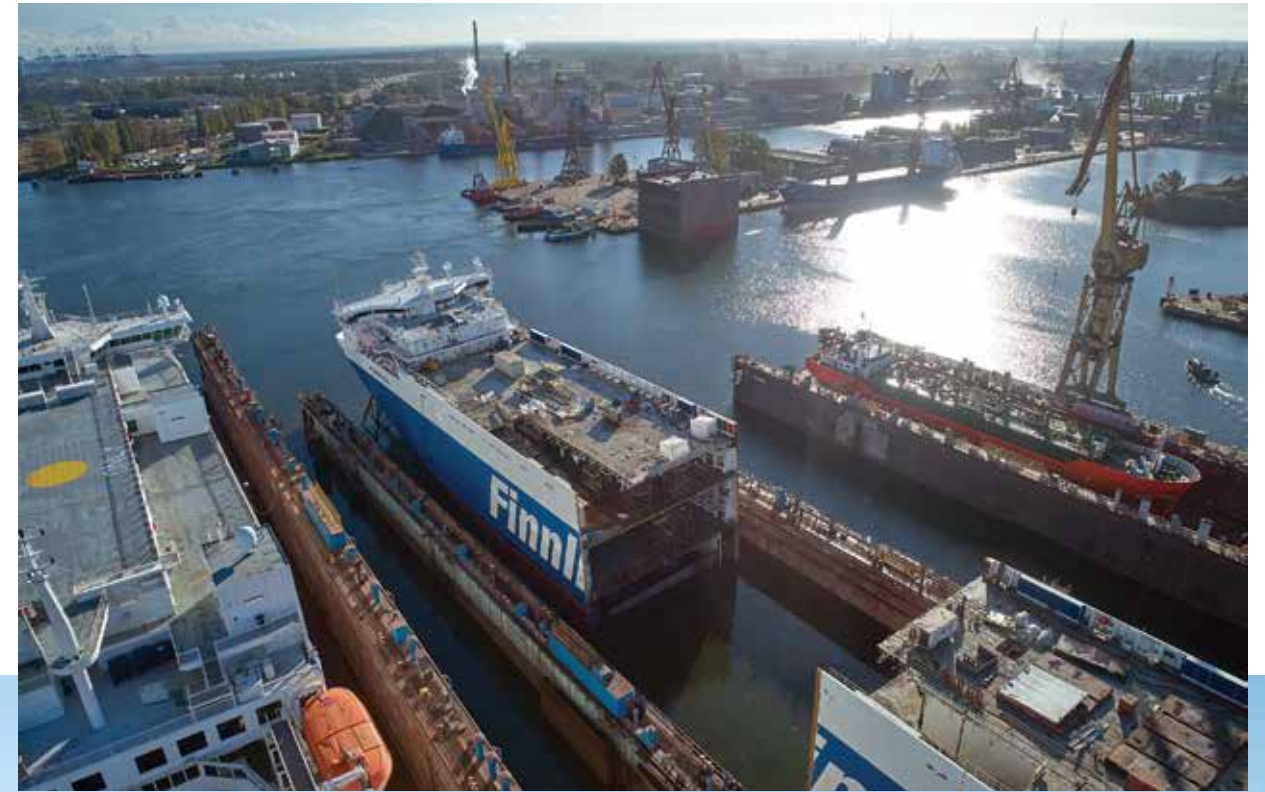
The hull in two pieces in the dock and the previously fabricated insert, in the background. Photo: Cezary Gierszewski/5XMEDIA
