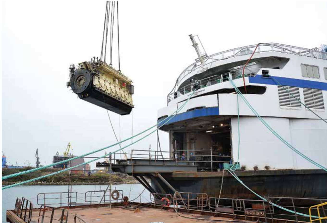
The old engines were removed from the vessel using the REM 220 floating sheerleg. Photo: Sławomir Lewandowski
