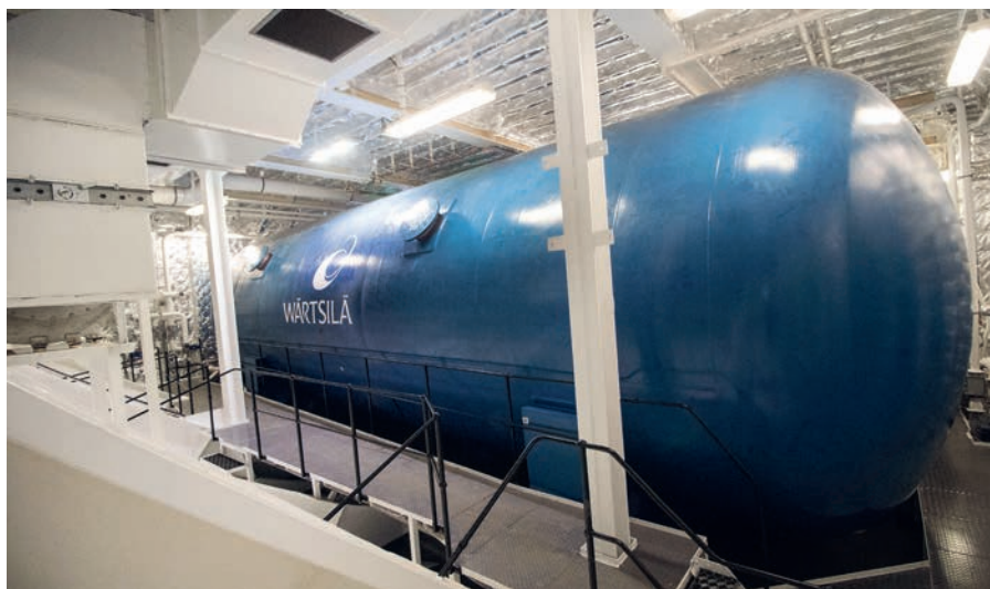
The new cryogenic tank on-board the ferry. Photo: Sławomir Lewandowski
