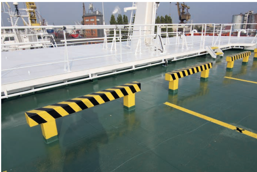
The new trailer deck has been fitted with wheel stops/parking blocks.
