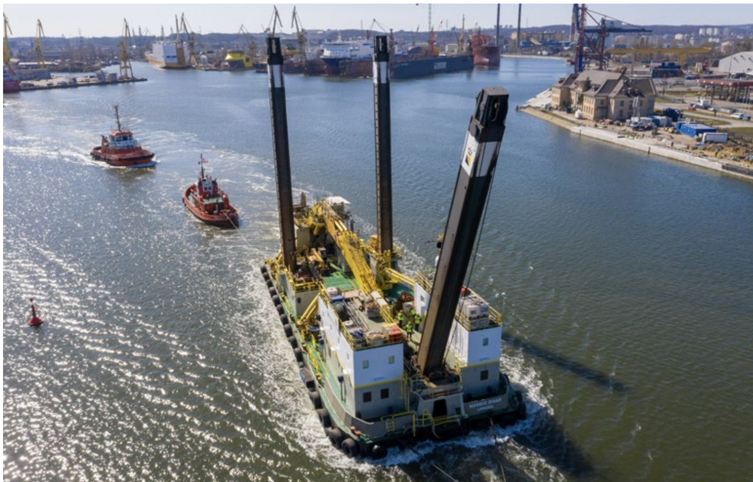
The Nordic Giant backhoe dredger after repair departing from our yard with the assistance of tugs. Photo: Marcin Koszałka
