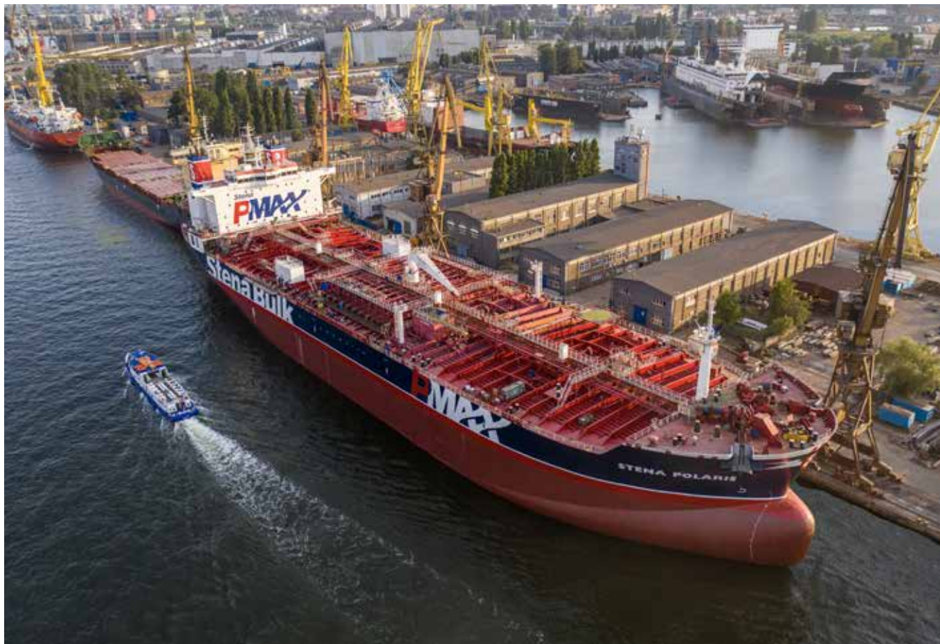
Stena Polaris with the BWT system installed in two deckhouses (the white casings visible on the main deck) at Remontowa.
