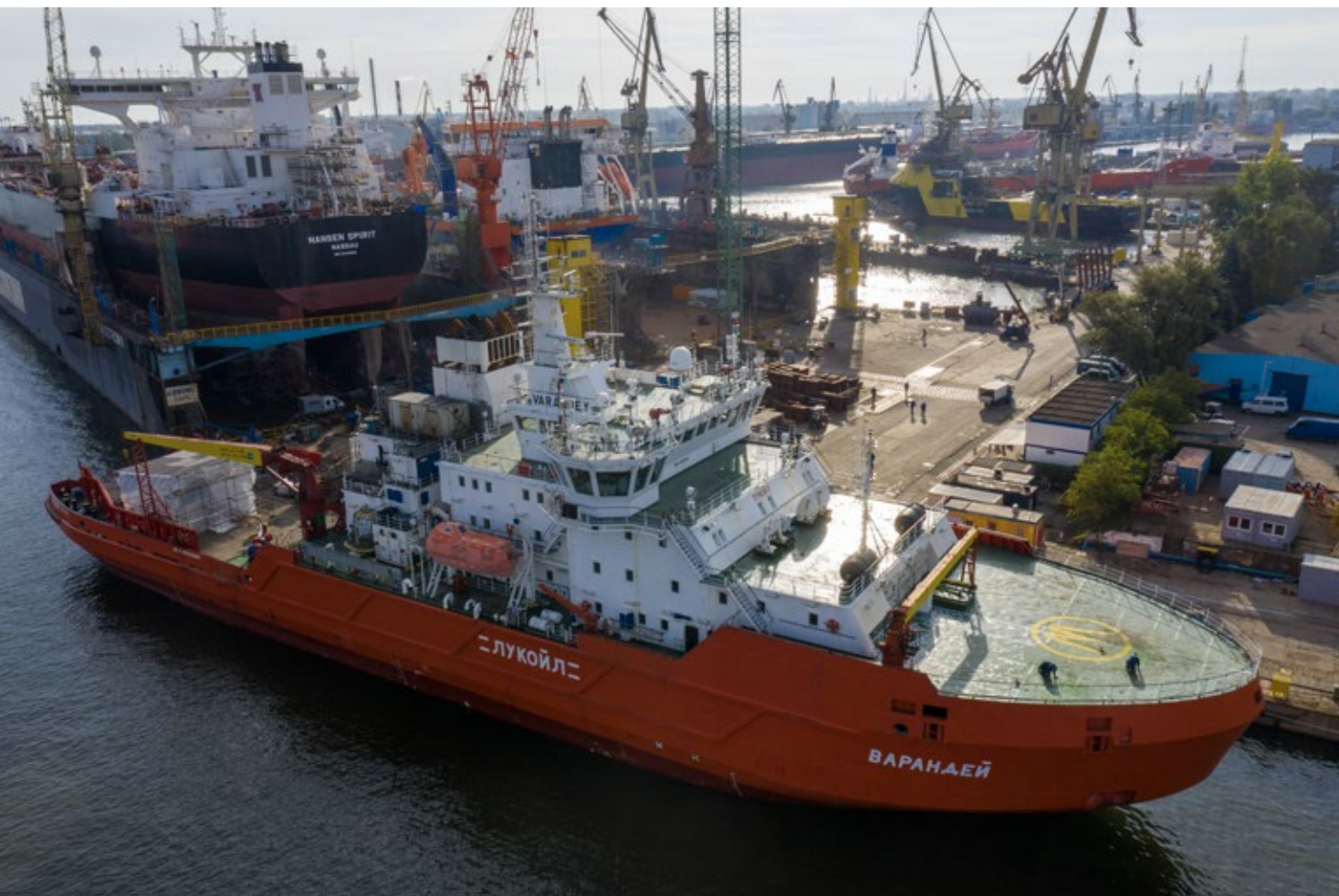
Varandey at Remontowa. The arctic icebreaker is capable of cutting through solid ice over 1.5 metres thick and can operate in extreme temperatures as low as -45 degrees Celsius.
