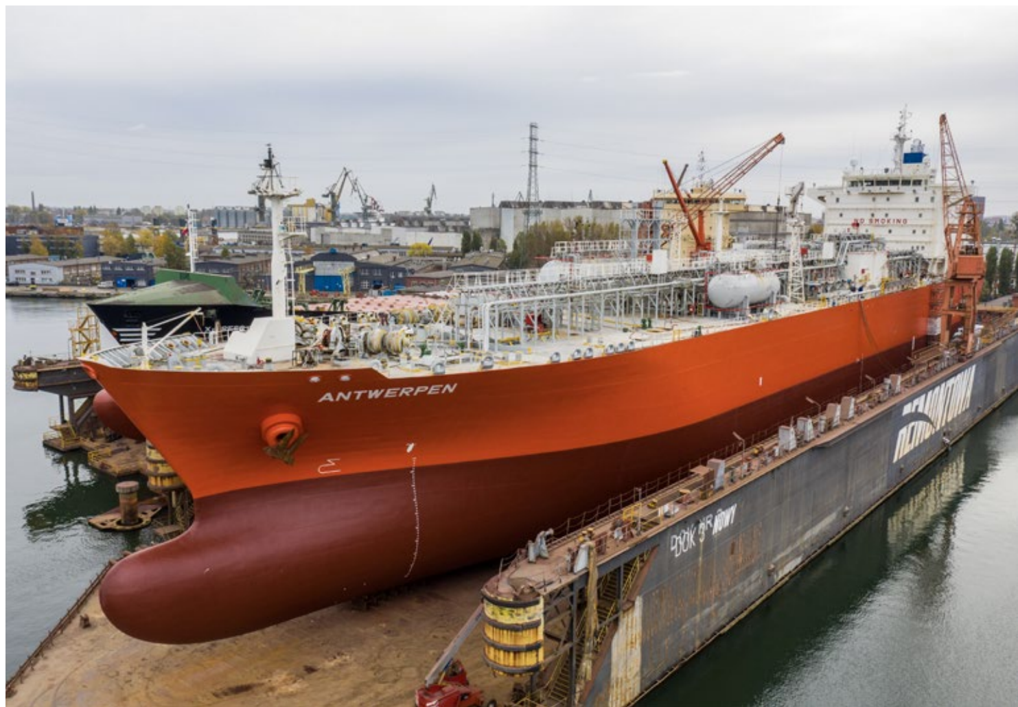
Antwerpen has been retrofitted with a Ballast Water Treatment System at Remontowa. Photo: Marcin Koszałka
